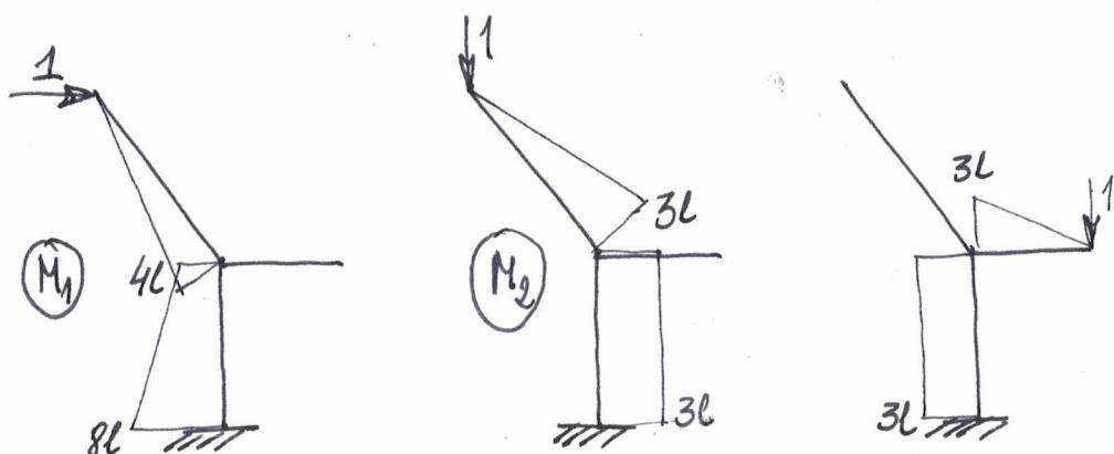
$$\begin{aligned} d_{11} &= 176 \frac{l^3}{EI} \\ d_{12} &= -92 \frac{l^3}{EI} \\ d_{13} &= 72 \frac{l^3}{EI} \\ d_{22} &= 51 \frac{l^3}{EI} \\ d_{23} &= -36 \frac{l^3}{EI} \\ d_{33} &= 45 \frac{l^3}{EI} \end{aligned}$$
