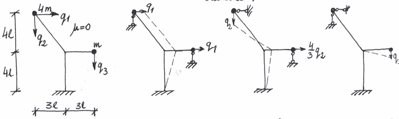
$$E_k = \frac{1}{2} \left( 4m \cdot (\dot{q}_1^2 + \dot{q}_2^2) + m \cdot ((\dot{q}_1 + \frac{4}{3}\dot{q}_2)^2 + \dot{q}_3^2) \right) = \frac{1}{2} \cdot m \left[ 5\dot{q}_1^2 + \frac{16}{3}\dot{q}_1\dot{q}_2 + \frac{52}{9}\dot{q}_2^2 + \dot{q}_3^2 \right]$$
